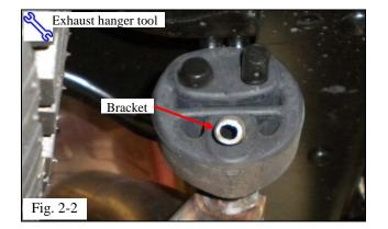
(b) Pry the passenger side tailpipe bracket loose from the rubber hanger (Fig. 2-2).
