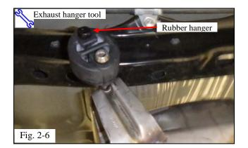
(g) Pry the rubber hanger located at the back of the muffler loose from the vehicle side hanger rod (Fig. 2-6).
